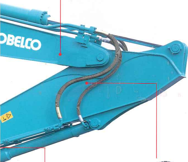
Integrated cast steel boom top
